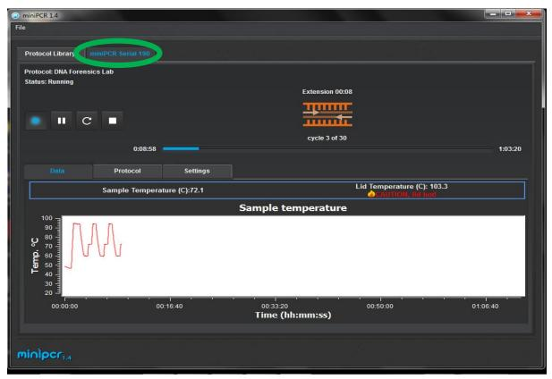
The miniPCR $^{TM}$  software allows each lab group to monitor the reaction parameters in real time, and to export the reaction data for analysis as a spreadsheet.
