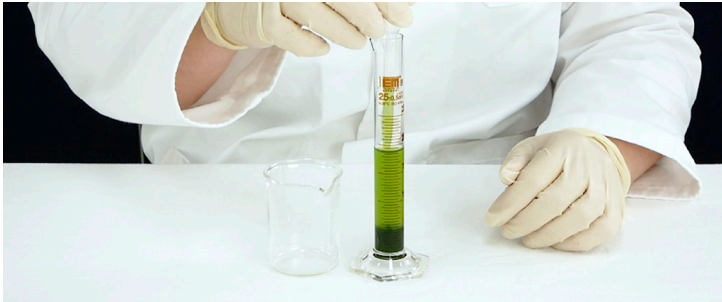
Figure 1: Supernatant separated from "plug" of dense algae
